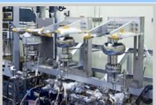
The single-cell ICHIRO cavities that achieved an accelerating gradient in excess of 50 mV/m.
