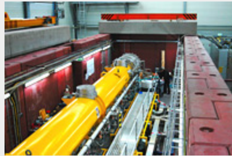
A brand-new test stand at DESY puts complete modules under the test. The performance of the module, its cavities, couplers and cables can be examined in great detail.
