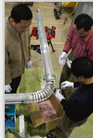
Scientists from China, working on assembly of liq-He transfer tube for STF at KEK.
