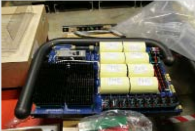
One of the Marx modulator cells, awaiting installation. (Photo: Calla Cofield)
