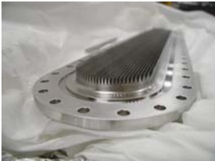
This insert, manufactured by SLAC and the company EMEGA, was placed inside the KEK-B accelerator beam pipe to trap stray electrons with its triangular grooves. (Photo by Mauro Pivi. Click for larger image.)
