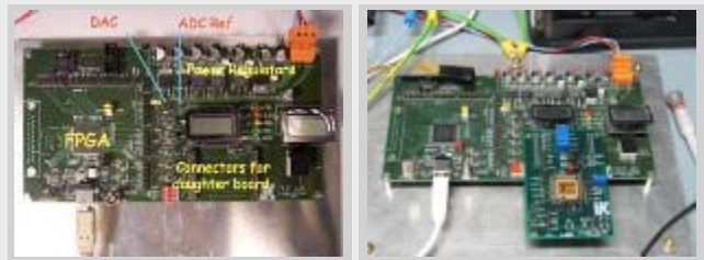
The generic motherboard designed at LPC to test the analogue-to-digital converter. Left with and right without ADC prototype.
