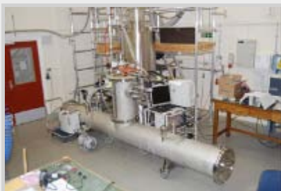
Where positrons are made: the undulator cryomodule for the positron source during tests at Rutherford Appleton Lab in the UK.
