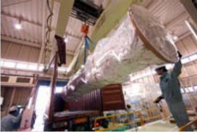
Italian made cryomodule being taken out from the container at Superconducting radiofrequency Test Facility (STF) at KEK.
