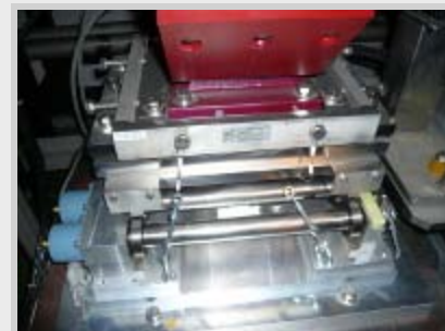
The quadrupole magnet sits on the mover. One of the wires was cut. The earthquake-proof apparatus worked as designed.
