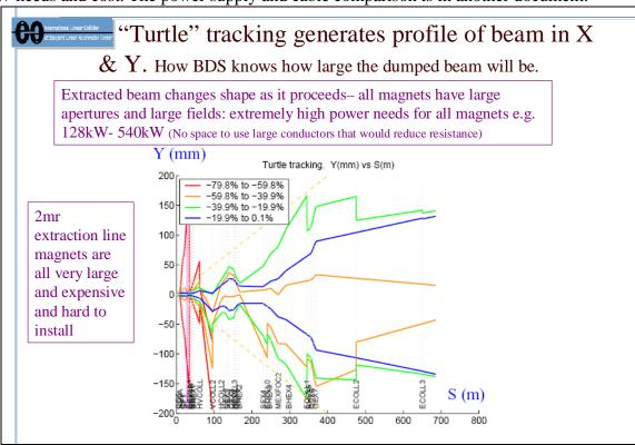
Figure 11: Overview of the extracted 2mr beam's Y dimension, leading to very large magnets.
