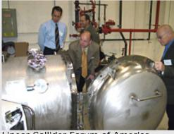
Linear Collider Forum of America members inspect a horizontal test cryostat at a Fermilab ILC test area.
