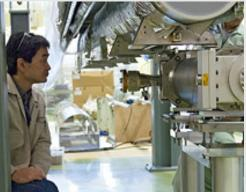
Norihito Ohuchi watching the crew align the position of the support ribs for a 9-cell cavity during assembly work of the STF (Superconducting RF Test Facility) cryomodule at KEK. (Image courtesy of N. Toge)
