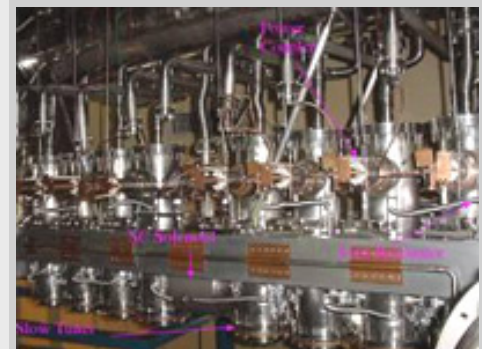
SCRF Cavity inside a Cryomodule installed in a beam line at Inter University Accelerator Center, Delhi.
