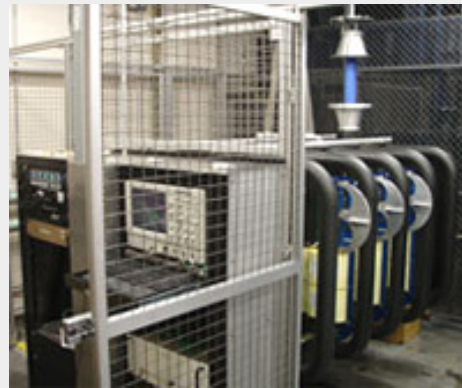
The prototype Marx modulator, designed and constructed at SLAC.
