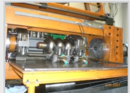
Perfect shape: a few hours earlier, this three-cell part of a cavity was just a niobium tube with two grooves.
