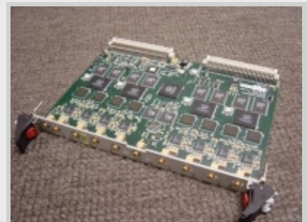
The Echotek boards that Fermilab and SLAC are installing in KEK's ATF damping ring.
