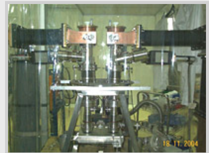
Pair of couplers, ready for tests in the LAL HF test stand.
