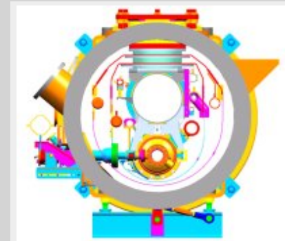
ILC cryomodule cutaway view
