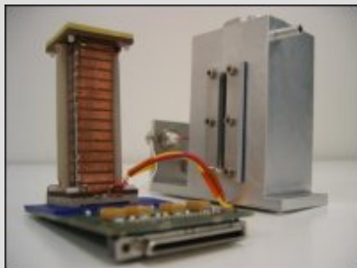
The mini TPC chamber which was used at Saclay to test the new Timepix chips.
