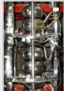
Cornell's re-entrant nine-cell cavity was tested with the second-sound method. The yellow dot shows where a quench occurred.
