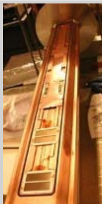
A retarding field analyser for electron cloud measurements in wiggler chambers.
