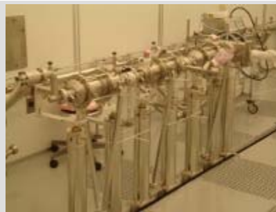
The assembled three-cavity string for the third-harmonic cryomodule.
