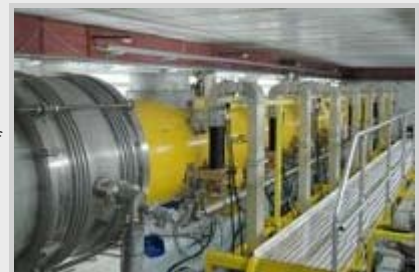
The cryomodule that set the world gradient record in the testbench at DESY
