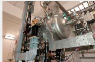
Engineers recently cooled this SRF test unit to 2 degrees Kelvin, or minus 271 degrees Celsius
