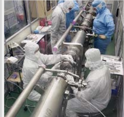
String assembly of DESY and Fermilab cavities for the S1 global experiment on Day 3: assembling the two DESY cavities, Z109 and Z108, with standard-length bellows. Image: Nobu Toge
