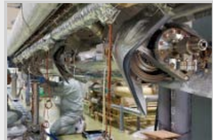
European made cavities, Z109 and Z108, with bottom portions of the magnetic shields. Image: Nobu Toge
