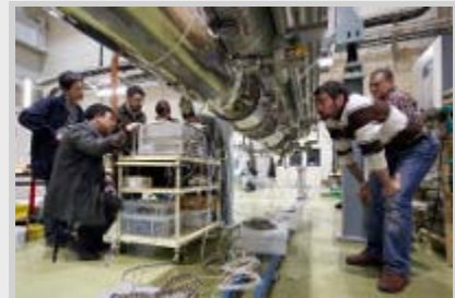
Test operation of the frequency tuner on U.S made cavity, AES004 for S1-global. from left: Norihito Ouchi (KEK), Yasuchika Kirk Yamamoto (KEK), Carlo Pagani (INFN), Serena Barbanotti (Fermilab), Eiji Kako (KEK), Rocco Pararella (INFN), Angelo Bosotti (INFN). Image: Nobu Toge
