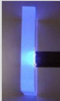
Blue light emitted by a piece of plastic scintillator. Image: Frank Simon.
