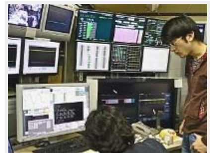
The ATF control room at KEK, Japan, where the Shintake monitor group (University of Tokyo) is analysing the online data for the beam size measurement. The measured fringe pattern can be seen in a monitor. Image: KEK
