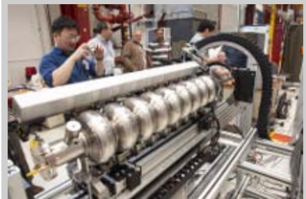
Full view of the KEK cavity tuning machine.
