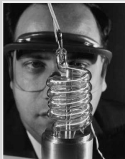
Theodore Maiman with the first working laser at Hughes Research Laboratory in 1960 Photo Credit: HRL Laboratories, LLC, from laserfest.org website
