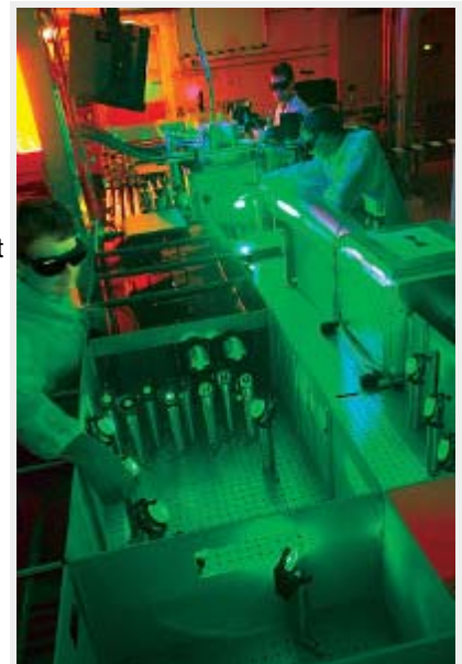
The laser used to accelerate electrons by plasma-wakefield acceleration to one billion electron volts in only three centimetres. (From Symmetry Magazine October 2009 – Image: Roy Kaltschmidt, Lawrence Berkeley National Laboratory)
