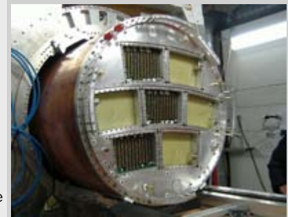
Many different institutes and labs in Germany are involved in the development of a time projection chamber (TPC) for the ILD detector.
