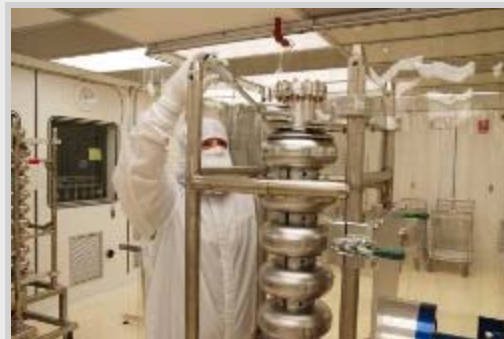
Fermilab technician Jim Folkie, under the training of Rongli Geng, performs a nine-cell cavity assembly in the Jefferson Lab clean room. The Jefferson Lab team has developed a specific procedure for assembling a superconducting radiofrequency cavity, including prescriptions for its orientation and the order in which parts are put together. The whole operation is designed to minimise contamination. Image: Rongli Geng
