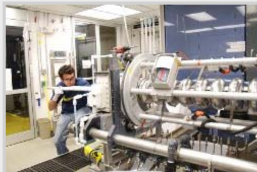
Jefferson Lab technician James Davenport carefully inserts a cathode into an ILC nine-cell cavity for the electropolishing process. Successful placement of the cathode requires a steady hand since the cavity aperture is very small. Image: Rongli Geng
