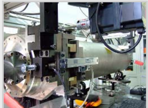
Test setup for an active tuner, built by the IHEP group, which has been attached to a cavity package in use and on lease from KEK. Photo: Nobu Toge
