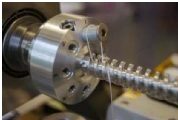
Daresbury and Rutherford-Appleton laboratories' helical superconducting undulator at the beginning of a winding. Wires arranged are around the beam tube like stripes on a barber pole. This allows the photons to be circularly polarised, which can then produce circularly polarised positrons. Image:
