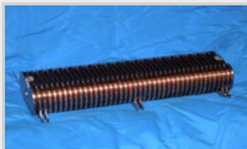
An early, 42-magnetic-pole test coil of Argonne National Laboratory's planar superconductor undulator. A planar undulator has two cores, each wound with superconducting wire, which are placed on opposite sides of the electron beam. The electron wiggles will lie in a plane, and the resulting photons will be linearly polarised. Image: Yury Ivanyushenkov
