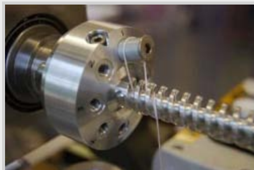
Daresbury and Rutherford-Appleton laboratories' helical superconducting undulator at the beginning of a winding. Wires arranged are around the beam tube like stripes on a barber pole. This allows the photons to be circularly polarised, which can then produce circularly polarised positrons. Image: Jim Clarke
