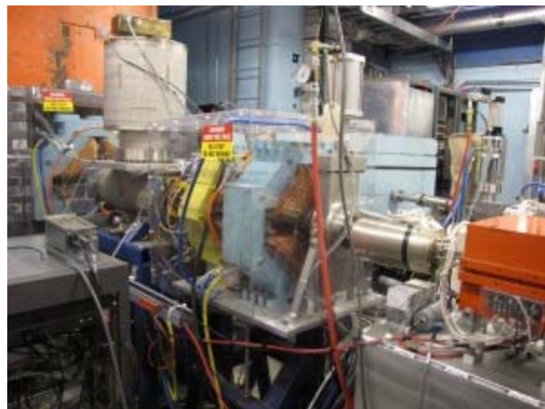
Part of the beam diagnostics system of the Energy Recovery Linac injector prototype.
