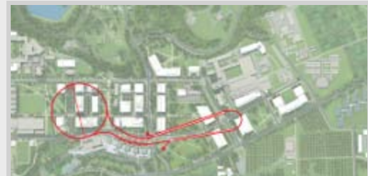
Cornell's Energy Recovery Linac will lie under the Cornell campus. The Cornell Electron Storage Ring, known as CESR, will be incorporated as part of the ERL. Image provided courtesy of Bruce Dunham.
