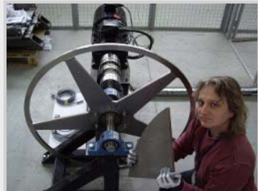
Ian Bailey holds one of the wheel's off-cuts next to the rotating positron target prototype. Off-cuts are used for wheel material studies. A motor sits behind the wheel. Image courtesy of Ian Bailey.
