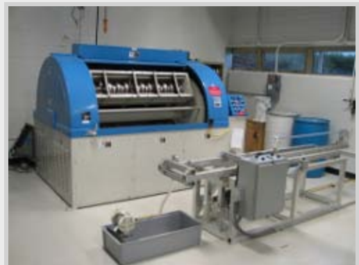
The tumbling machine (left) can hold two nine-cell accelerating cavities, rotating them up to 115 turns per minute. The rinsing device (right) washes the media out. Cavities must be absolutely free of any extraneous material after tumbling.
