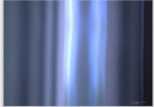
A mirror-like finish was achieved on a single-cell cavity after the tumbling process.
